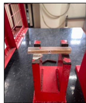
Fig. 6: Position of Test Sample on the Charpy Machine Base
