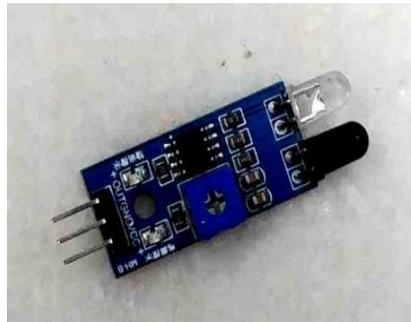
**Fig. 3: Infrared sensor**
