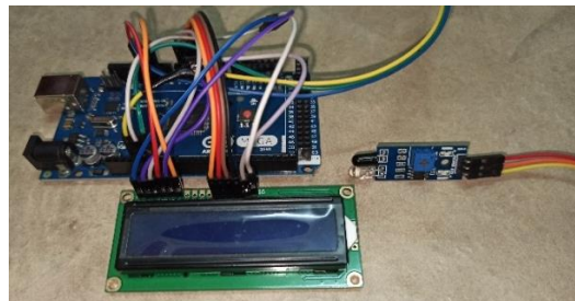
Fig. 7: Connection of the system
