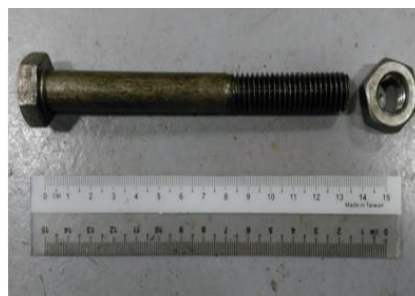
Fig. 3: Grade class of 4.6 bolt and nut
